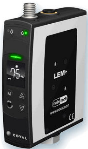
(a) Compact, High Flow Vacuum Pump, LEM+ Series, 85% max. vacuum, 2.5 mm nozzle ID, vacuum controlled 24 V DC NC and controlled blow-off 24V DC NC, electronic vacuum switch, 1 x M12 connector 5 pins, with Powerfull Blow-off.
