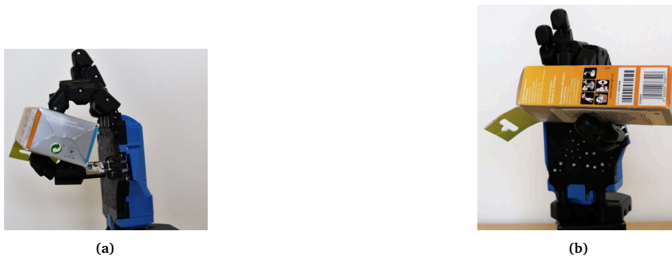
Figure 8: A pinch grasp of a smaller part from the Darko set of objects.
