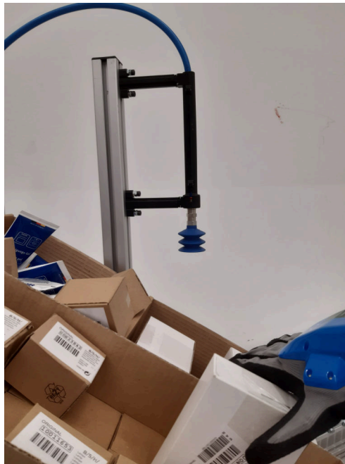
Figure 15: The hand tool attached to the shelf structure to a pair of brackets by means of magnets.
