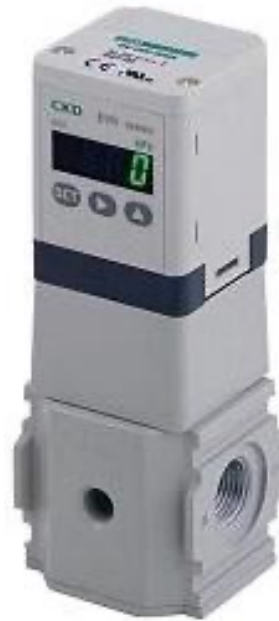
(b) Pressure regulator series EVD3900-0-10G-AP-B3-3, powered at 24 V DC, maximum pressure 900 kPa, input voltage range between 0 and 10 V, pneumatic port size G3/8, output voltage range between 0 and 5 V, error (PNP), B-type bracket, floor mounted.
