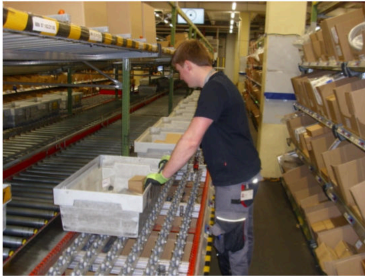
Figure 1: DARKO lead use case. Parts of varying shapes, weights and packaging are stored in boxes or trays on slanted shelves (see on the right of the picture).
